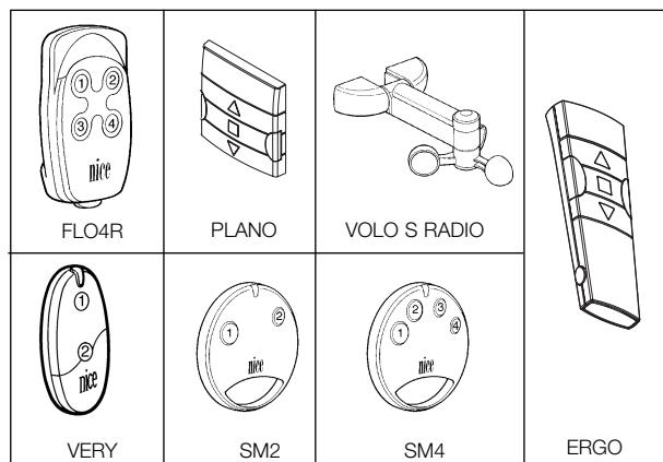
The transmitters have different kinds of coding, and the control unit is unable to recognise them simultaneously. The first transmitter memorised will thus determine the type of coding, and consequently the transmitters which can be memorised successively.
